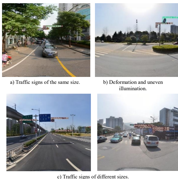
Figure 5. Detection results of ASFF&amp;SPP-YOLOv3 on TT100K dataset.
